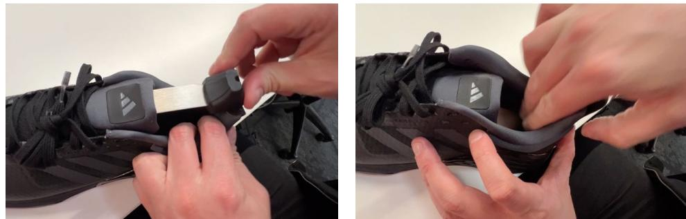
Ensure the USB cable is securely locked in between the guide of the heel counter and heel wall of the shoe, and not wrapped around the band.
