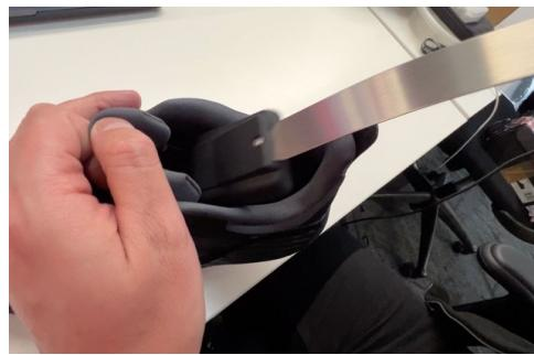
Push the heel counter forward and down into the heel of the shoe. This will flex the metal size band, creating tension in the band that will fix the heel counter in place.
